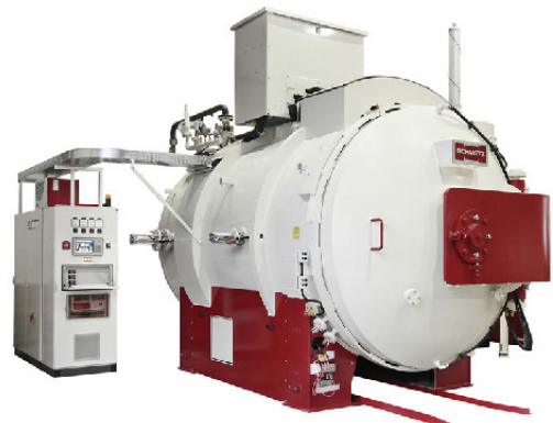
▲ WEIDER uses German SCHMETZ vacuum heat treatment technology
